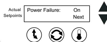
If no buttons are pressed, the display automatically returns to the Operating Screen after about fifteen seconds, saving the selection to memory.
