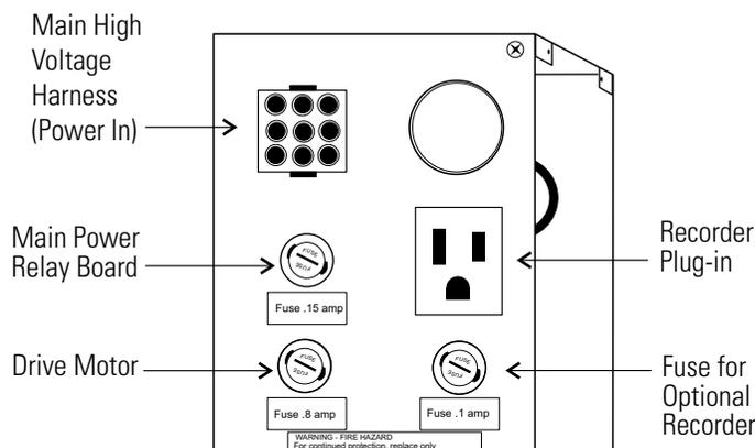
**Figure 4-3.** Fuse Holders and Connector Locations (Model SHKE436HP shown)
