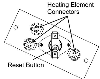
**Figure 4-8.** Connectors and Reset
