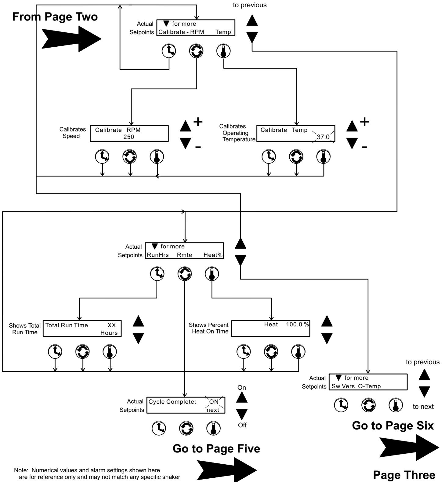
Note: Numerical values and alarm settings shown here are for reference only and may not match any specific shaker
