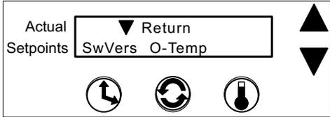
Press the Speed button beneath O-Temp and the screen at the right will appear, showing the temperatures being read by the Overtemperature sensor.
