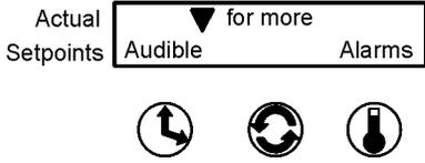
Then press the temperature button beneath Alarms.
