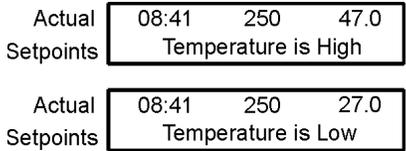
In the alarm state, the audible alarm is muted by pressing the Silence button, but rings back in about 15 minutes, if the alarm condition is still present. However, the message and indicator lights persist until the fault is corrected. Afterward, the remaining relevant alarm components are cleared by pressing the Silence button.
