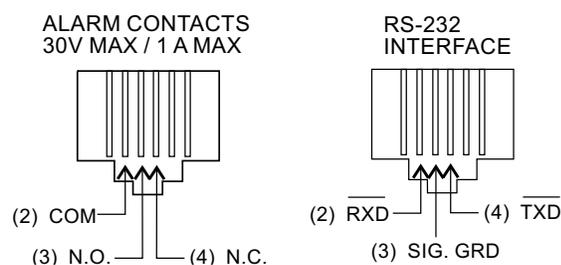
Figure 1-15. Remote Alarm and RS-232 Connectors
