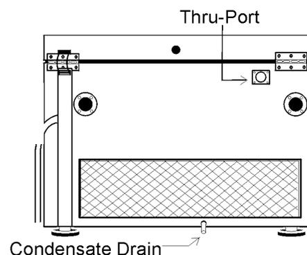
**Figure 1-5.** Drain Location
