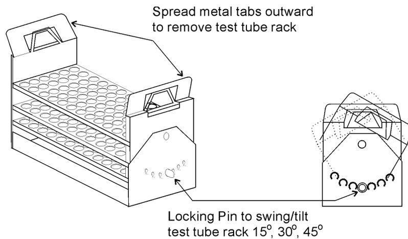
**Figure 1-13.** Test Tube Rack Holder
