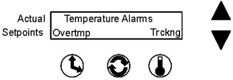
The following screen will appear and the present Temperature Tracking alarm limit setting will flash.
