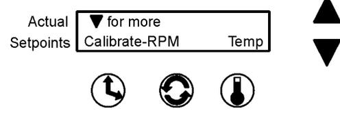
8. Using the up and down arrows, increase or decrease the temperature value to match the independent, accurate temperature measuring device.
