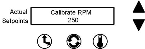
When finished, press any of the three buttons (Time, Speed, or Temp) to save the new setpoint value and return to the previous screen, or press nothing for about 15 seconds to save the new setpoint value and return to the Operating Screen.
