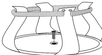
**Figure 1-11.** Clip Mounting Screw
