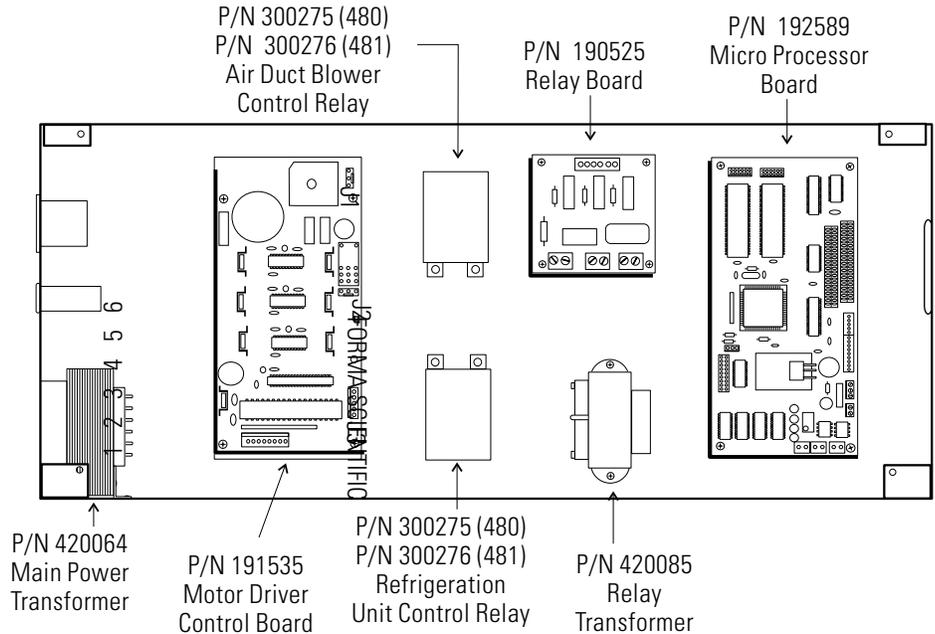
**Figure 4-4.** Electrical Component Locations, Relay Tray Compartment
