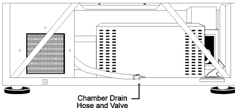
**Figure 1-4.** Chamber Drain Hose Location
