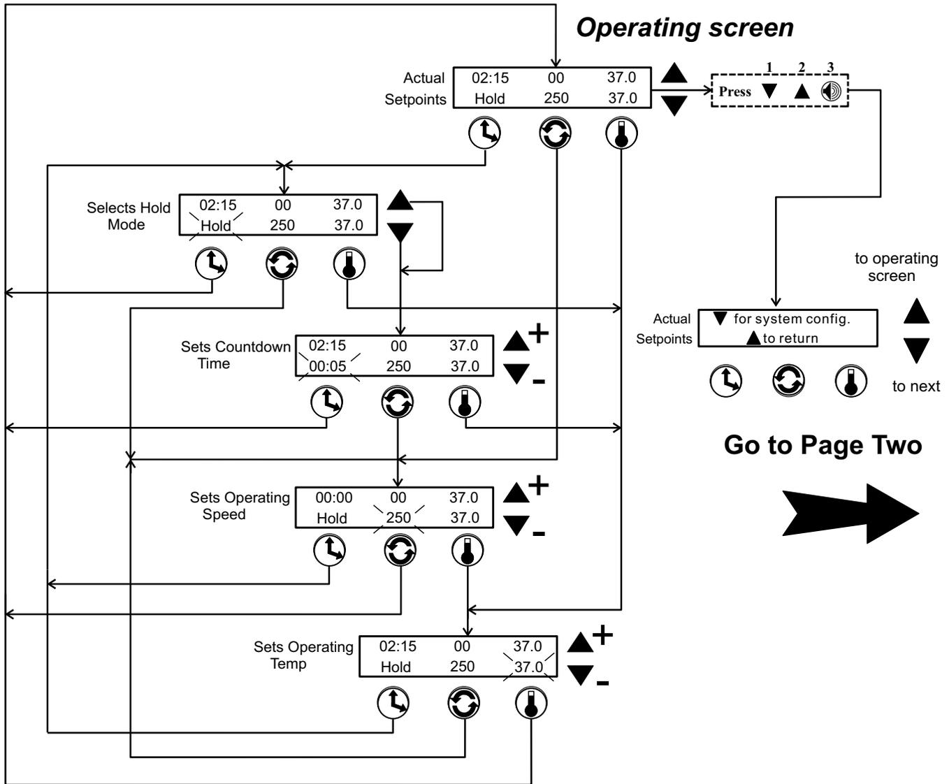
Note: Numerical values and alarm settings shown here are for reference only and may not match any specific shaker
