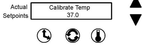
9. When complete, press the Time, Speed, or Temp button to save the setting. The display will return to the Calibrate - RPM Temp screen. (Or, if nothing is pressed for about fifteen seconds, the display will return to the Operating Screen and the setting will be automatically saved to memory.)
