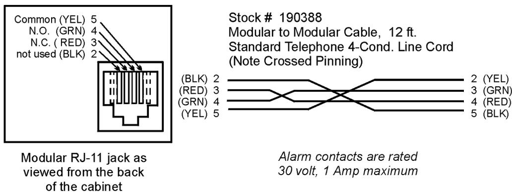
Figure 1-16. Remote Alarm Output to Screw Terminal Connection
