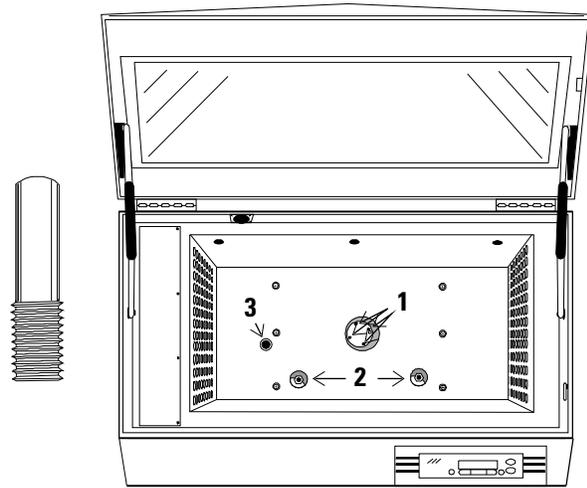
1) Platform mounting holes on drive mechanism (4)
