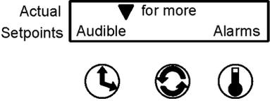
Then press the Time button beneath Audible. The screen at right appears.
