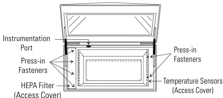
**Figure 4-1.** HEPA Filter and Temperature Sensors Locations
