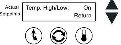
If no buttons are pressed, the display automatically returns to the Operating Screen after about 15 seconds, saving the selection to memory.
