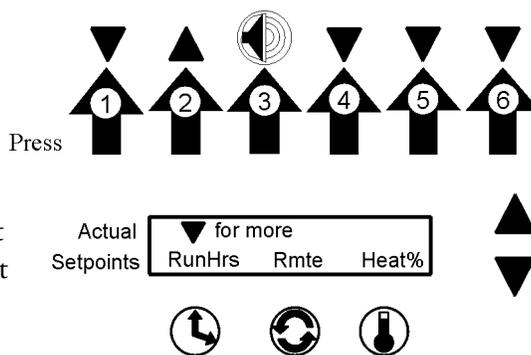
Press the Speed button beneath Remote (Rmte). The alarms will be shown in the following sequence.
