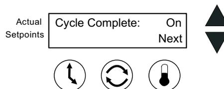
If no buttons are pressed, the display automatically returns to the Operating Screen after about 15 seconds, saving the selection to memory.
