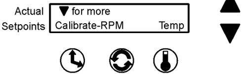
Then press the Speed button beneath RPM.
