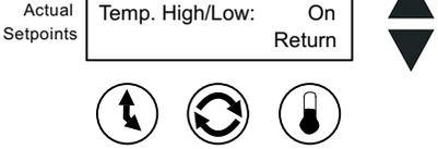
If no buttons are pressed, the display will automatically return to the Operating Screen after about 15 seconds, saving the selection to memory.
