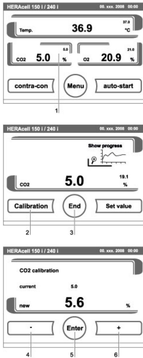
**Figure. 74.** CO<sub>2</sub> calibration procedure
