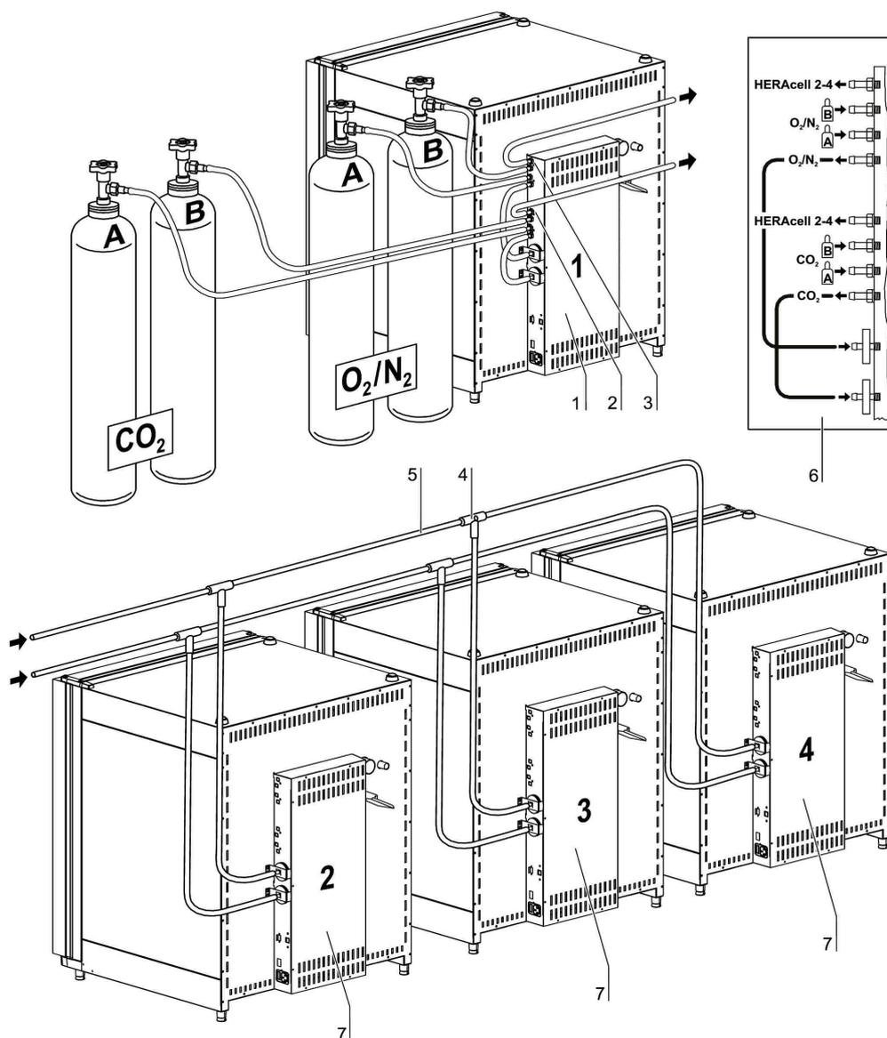
**Figure. 9.** Looped-through gas supply **HERACELL<sup>®</sup> 240i**
