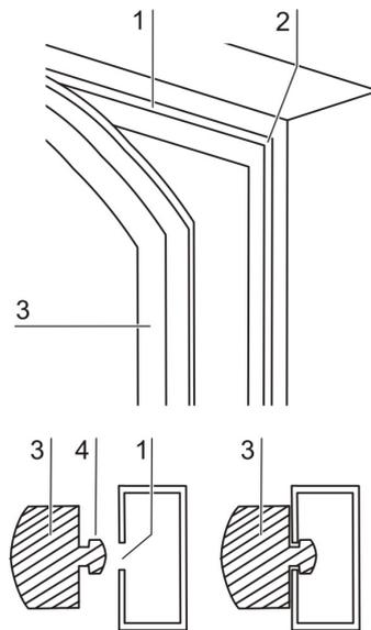
**Figure. 77.** Magnetic door seal replacement
