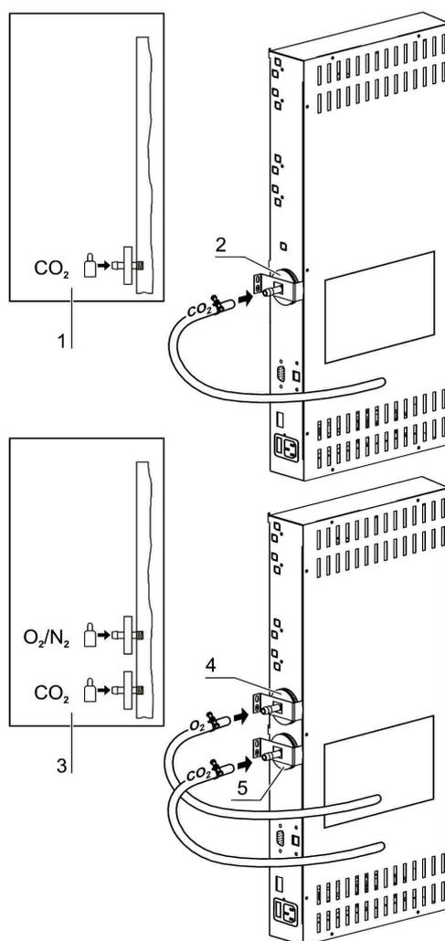
**Figure. 25.** Gas connection without gas monitoring system
