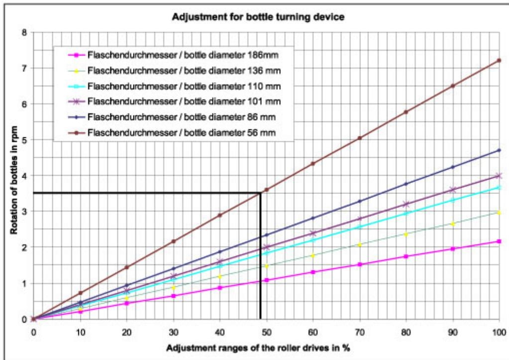
**Figure. 22.** Bottle turning speed
