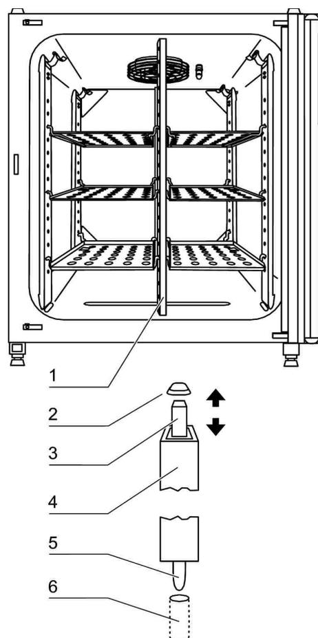
**Figure. 23.** Center strut installation
