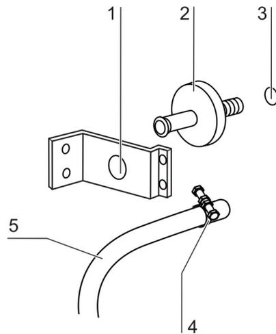
**Figure. 75.** Gas inlet filter installation
