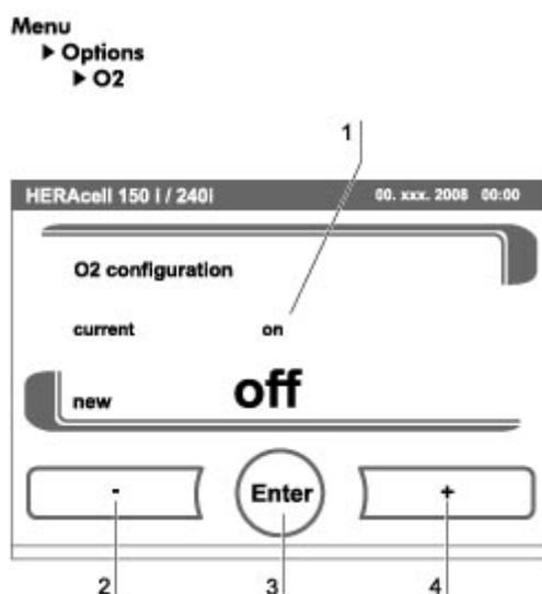
**Figure. 58.** Switching the O<sub>2</sub> control on and off
