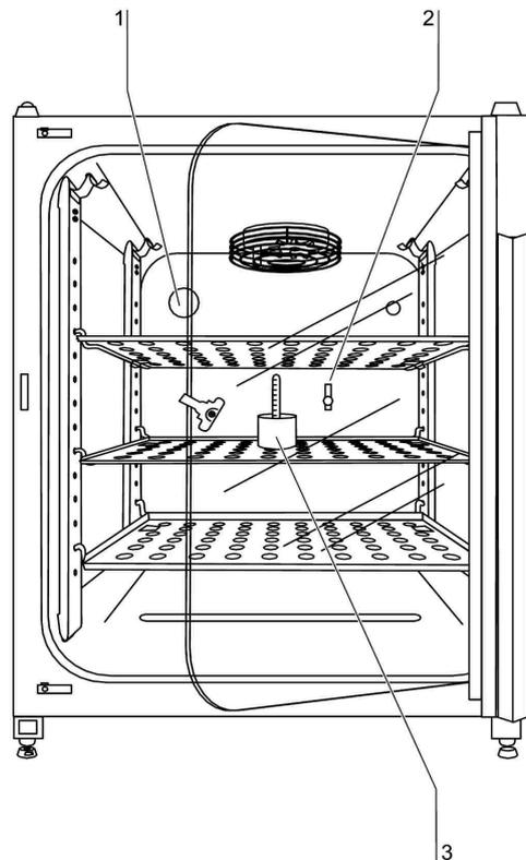
**Figure. 70.** Preparing the temperature calibration
