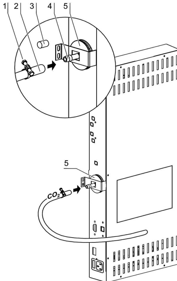
**Figure. 24.** Installing gas pressure hoses
