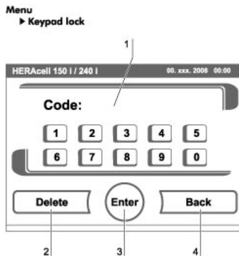
**Figure. 61.** Enabling/disabling the keypad lock
