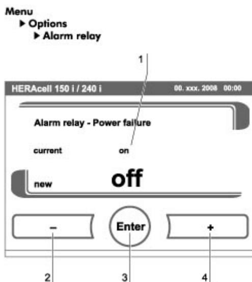
**Figure. 52.** Alarm relay setting
