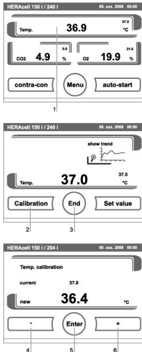
**Figure. 71.** Temperature calibration procedure
