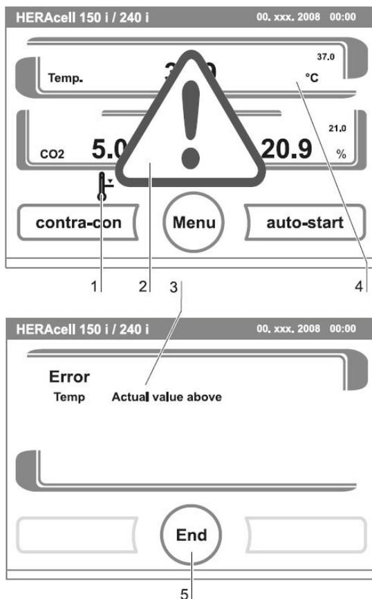
**Figure. 65.** Event error overtemperature
