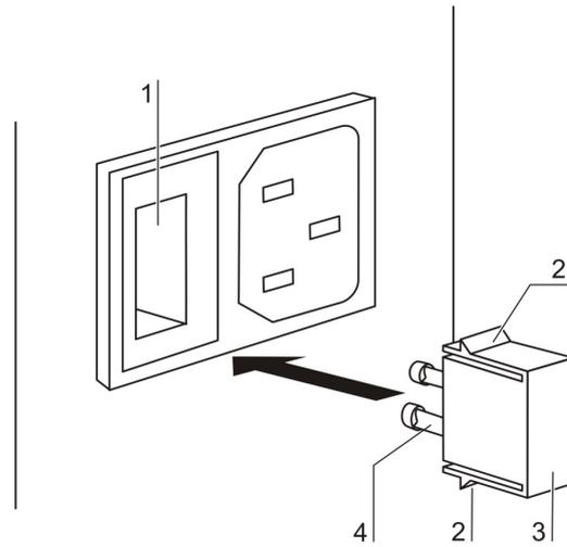
**Figure. 76.** Device fuse replacement
