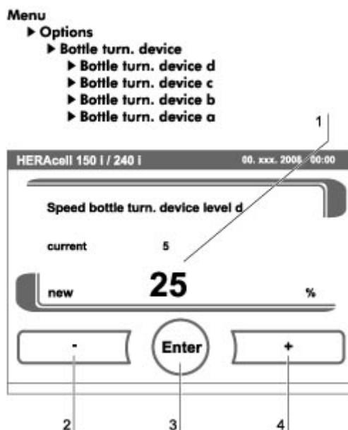
**Figure. 57.** Bottle turning device speed setting
