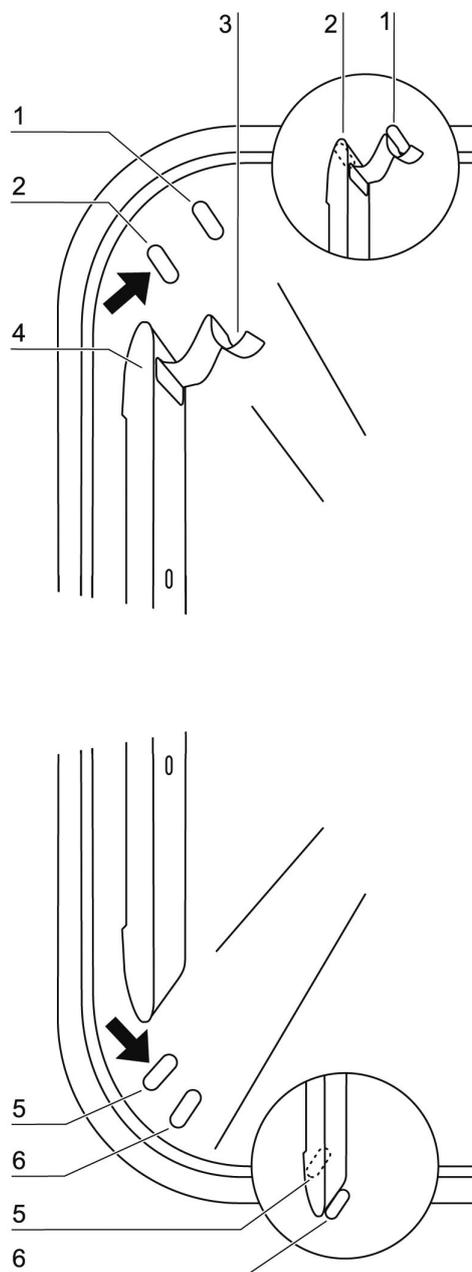
**Figure. 18.** Support rail installation/removal
