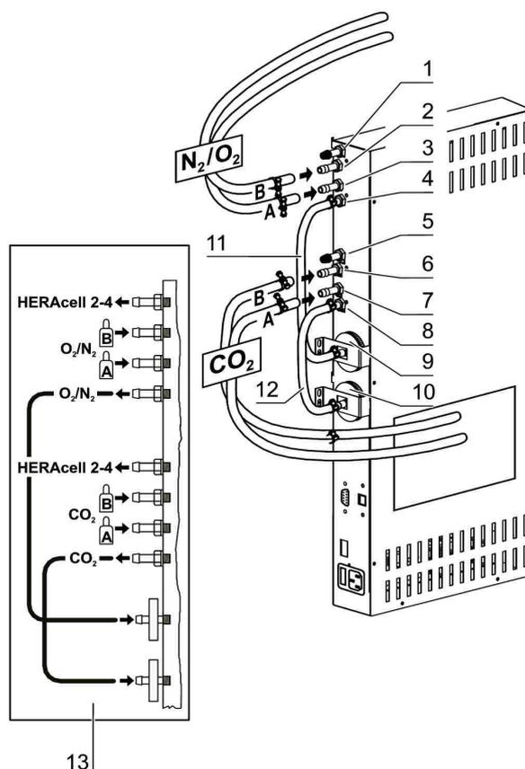
**Figure. 27.** Combined connection with gas monitoring system (optional)
